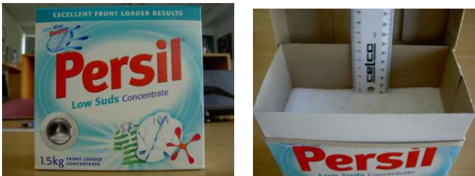
Example 2: Unavoidable settling –Laundry Powder
